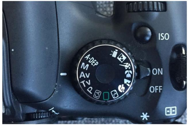
This mode, usually denoted by "A" or "Av", lets you change the aperture, and your camera will handle the rest. In general, this is used for controlling the depth of field in your photo.
